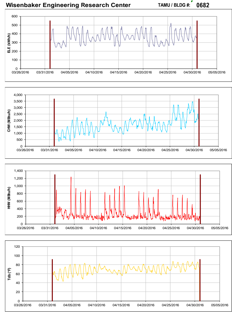
Figure III-116 Hourly Whole Building Electricity, Chilled Water, and Hot Water Consumption for Wisnaker Engineering Research Center during the Month of April 2016 and the Corresponding Hourly Outdoor Dry Bulb Temperature for College Station, TX
