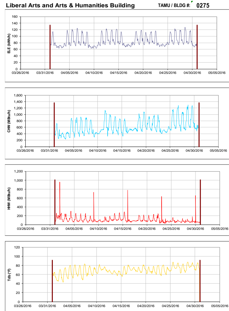
Figure III-2 Hourly Whole Building Electricity, Chilled Water, and Hot Water Consumption for Liberal Arts and Arts & Humanities Building during the Month of April 2016 and the Corresponding Hourly Outdoor Dry Bulb Temperature for College Station, TX
