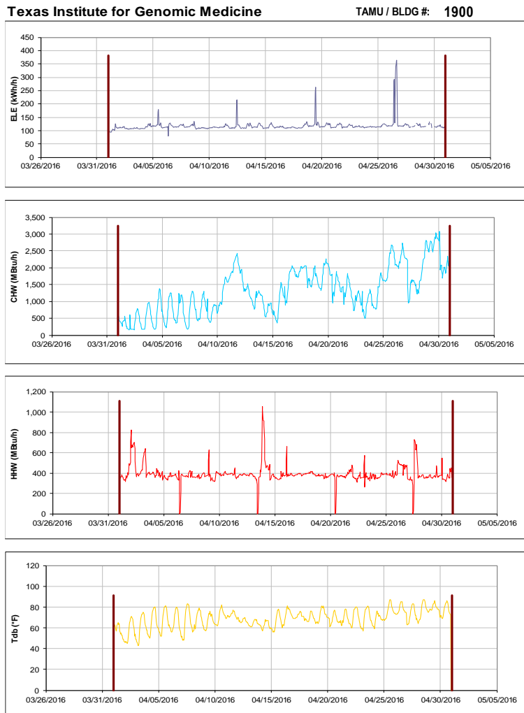
Figure III-183 Hourly Whole Building Electricity, Chilled Water, and Hot Water Consumption for Texas Institute for Genomic Medicine during the Month of April 2016 and the Corresponding Hourly Outdoor Dry Bulb Temperature for College Station, TX
