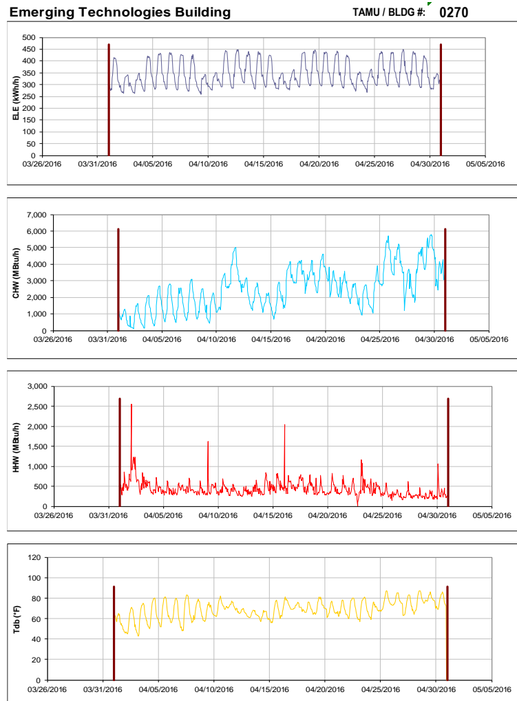
Figure III-1 Hourly Whole Building Electricity, Chilled Water, and Hot Water Consumption for Emerging Technologies Building during the Month of April 2016 and the Corresponding Hourly Outdoor Dry Bulb Temperature for College Station, TX
