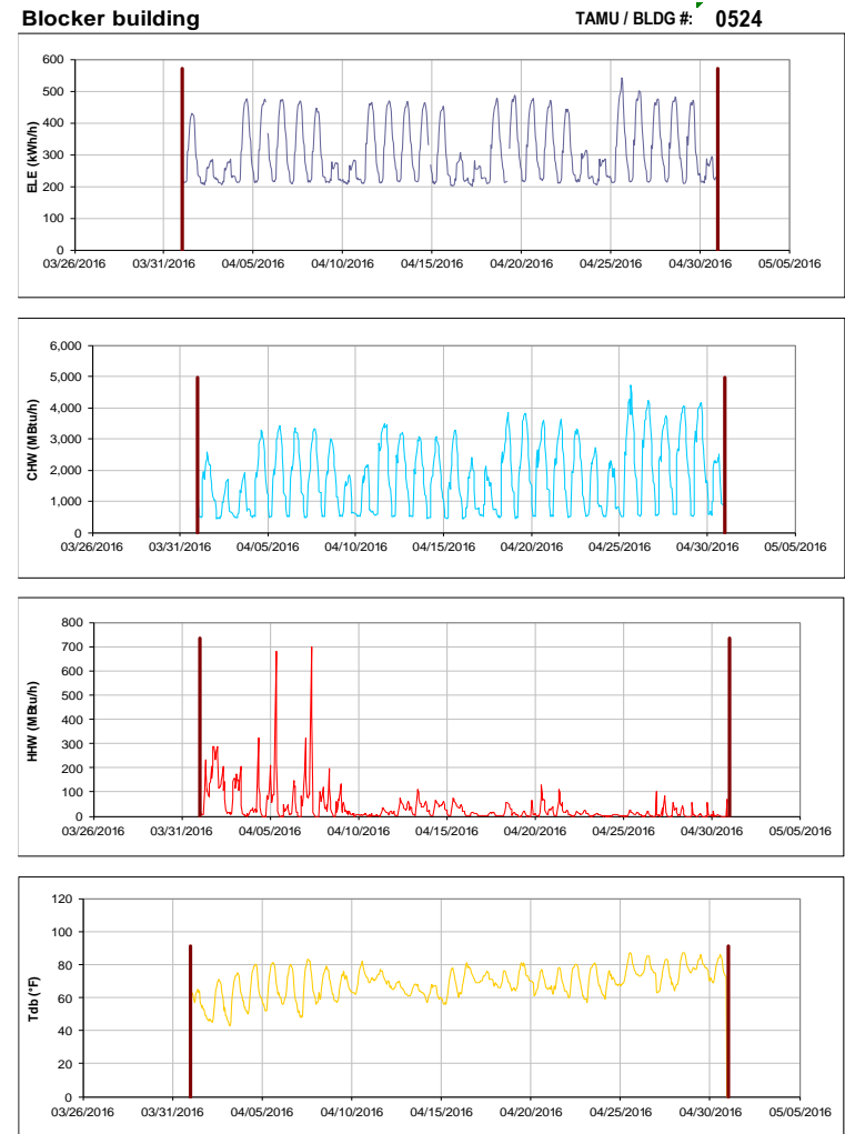
Figure III-110 Hourly Whole Building Electricity, Chilled Water, and Hot Water Consumption for Blocker building during the Month of April 2016 and the Corresponding Hourly Outdoor Dry Bulb Temperature for College Station, TX
