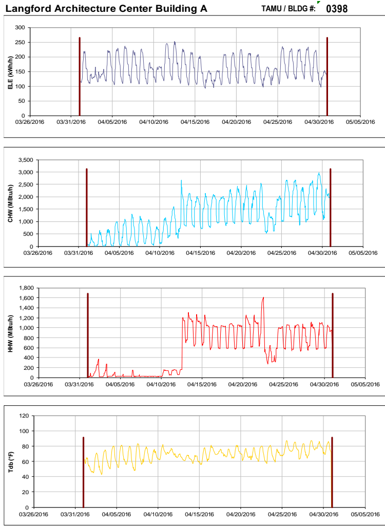
Figure III-25 Hourly Whole Building Electricity, Chilled Water, and Hot Water Consumption for Langford Architecture Center Building A during the Month of April 2016 and the Corresponding Hourly Outdoor Dry Bulb Temperature for College Station, TX
