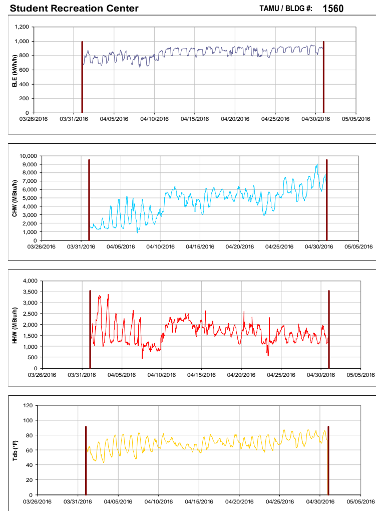
Figure III-168 Hourly Whole Building Electricity, Chilled Water, and Hot Water Consumption for Student Recreation Center during the Month of April 2016 and the Corresponding Hourly Outdoor Dry Bulb Temperature for College Station, TX
