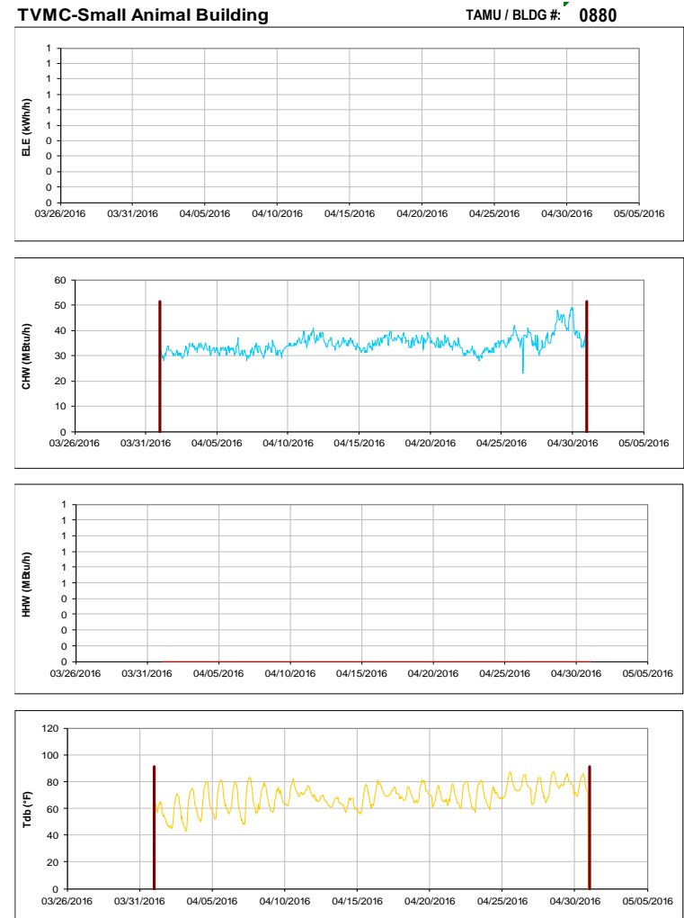
Figure III-120 Hourly Whole Building Electricity, Chilled Water, and Hot Water Consumption for TVMC-Small Animal Building during the Month of April 2016 and the Corresponding Hourly Outdoor Dry Bulb Temperature for College Station, TX
