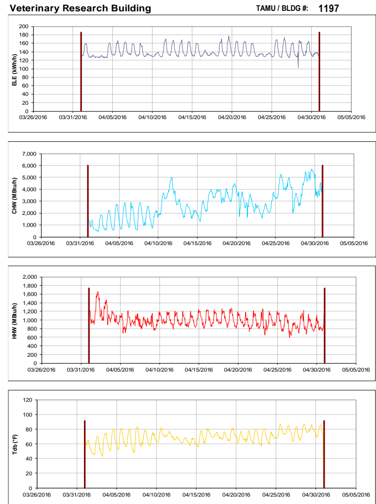
Figure III-130 Hourly Whole Building Electricity, Chilled Water, and Hot Water Consumption for Veterinary Research Building during the Month of April 2016 and the Corresponding Hourly Outdoor Dry Bulb Temperature for College Station, TX
