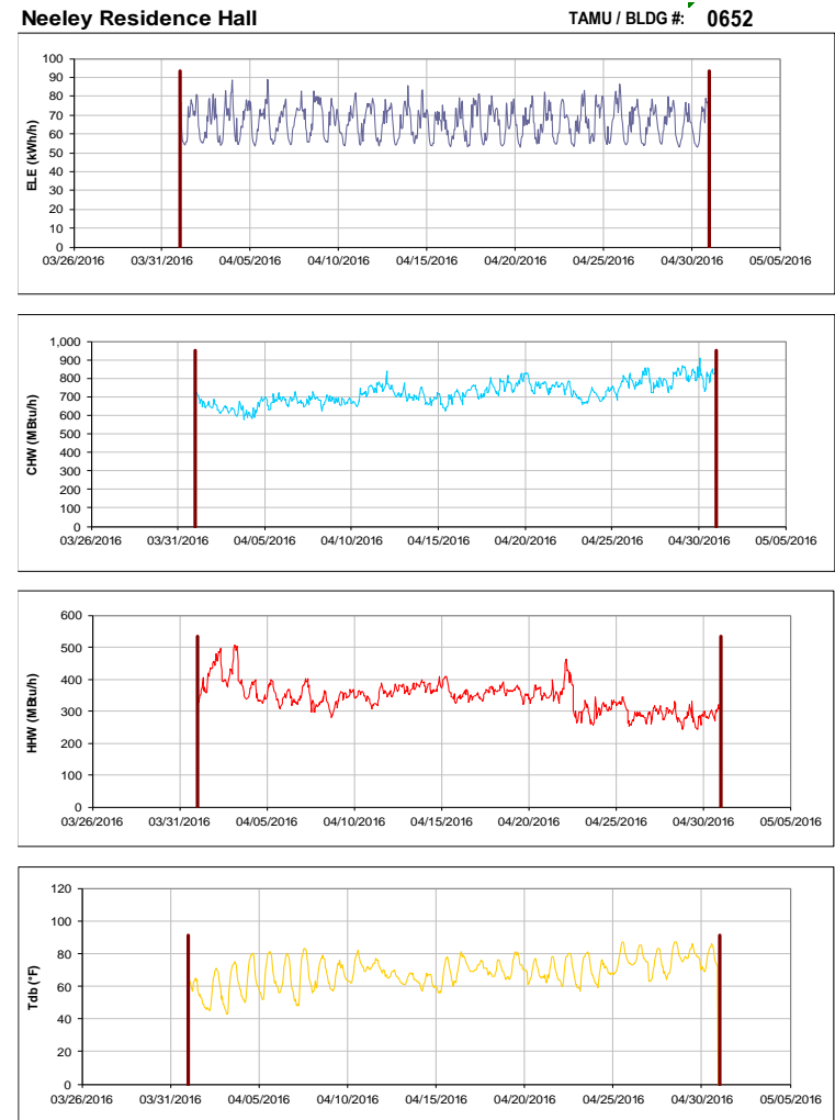
Figure III-114 Hourly Whole Building Electricity, Chilled Water, and Hot Water Consumption for Neeley Residence Hall during the Month of April 2016 and the Corresponding Hourly Outdoor Dry Bulb Temperature for College Station, TX
