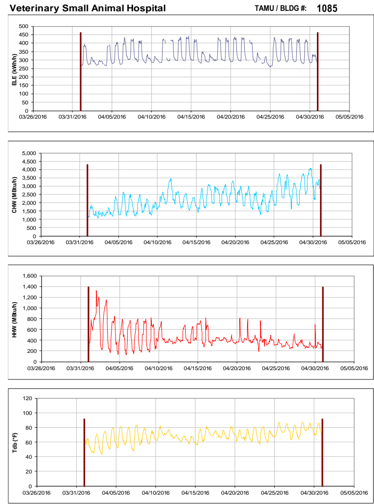
Figure III-124 Hourly Whole Building Electricity, Chilled Water, and Hot Water Consumption for Veterinary Small Animal Hospital during the Month of April 2016 and the Corresponding Hourly Outdoor Dry Bulb Temperature for College Station, TX
