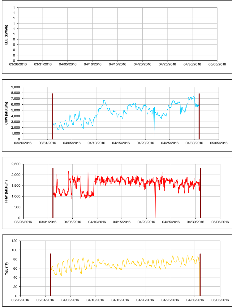
Figure III-187 Hourly Whole Building Electricity, Chilled Water, and Hot Water Consumption for NCTM Manufacturing Building during the Month of April 2016 and the Corresponding Hourly Outdoor Dry Bulb Temperature for College Station, TX
