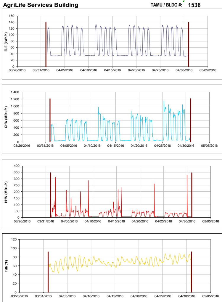
Figure III-161 Hourly Whole Building Electricity, Chilled Water, and Hot Water Consumption for AgriLife Services Building during the Month of April 2016 and the Corresponding Hourly Outdoor Dry Bulb Temperature for College Station, TX
