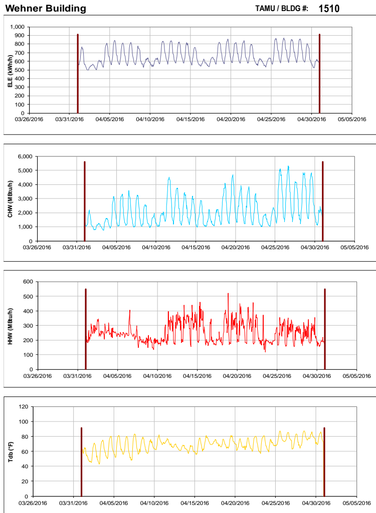
Figure III-153 Hourly Whole Building Electricity, Chilled Water, and Hot Water Consumption for Wehner Building during the Month of April 2016 and the Corresponding Hourly Outdoor Dry Bulb Temperature for College Station, TX
