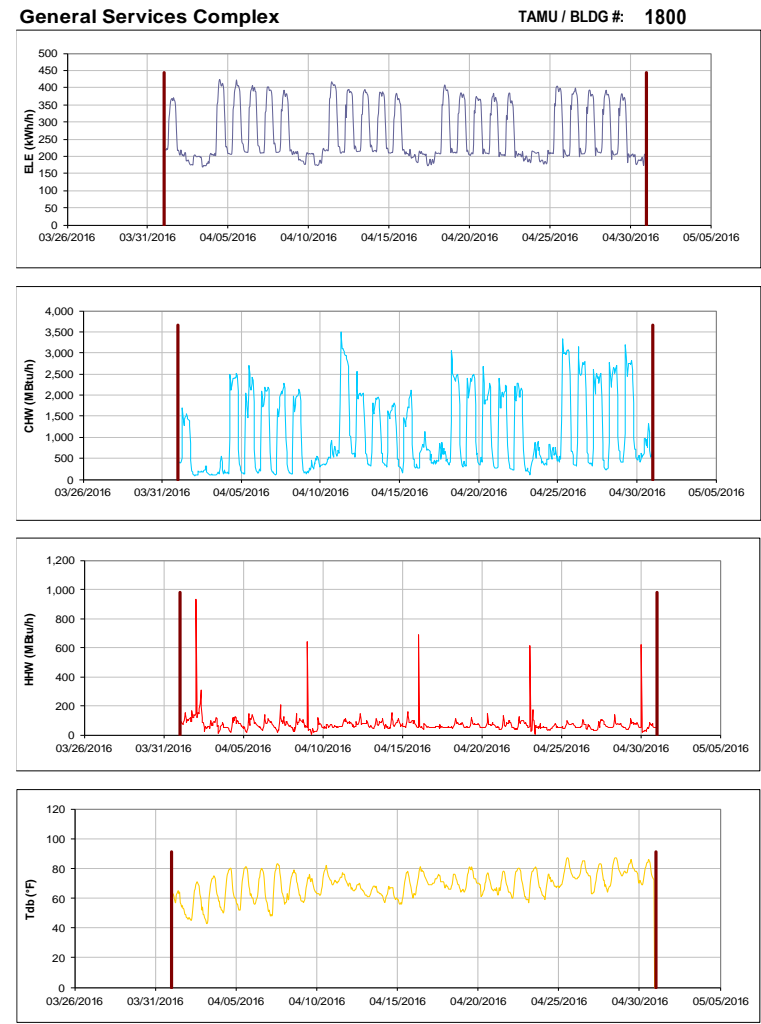
Figure III-180 Hourly Whole Building Electricity, Chilled Water, and Hot Water Consumption for General Services Complex during the Month of April 2016 and the Corresponding Hourly Outdoor Dry Bulb Temperature for College Station, TX
