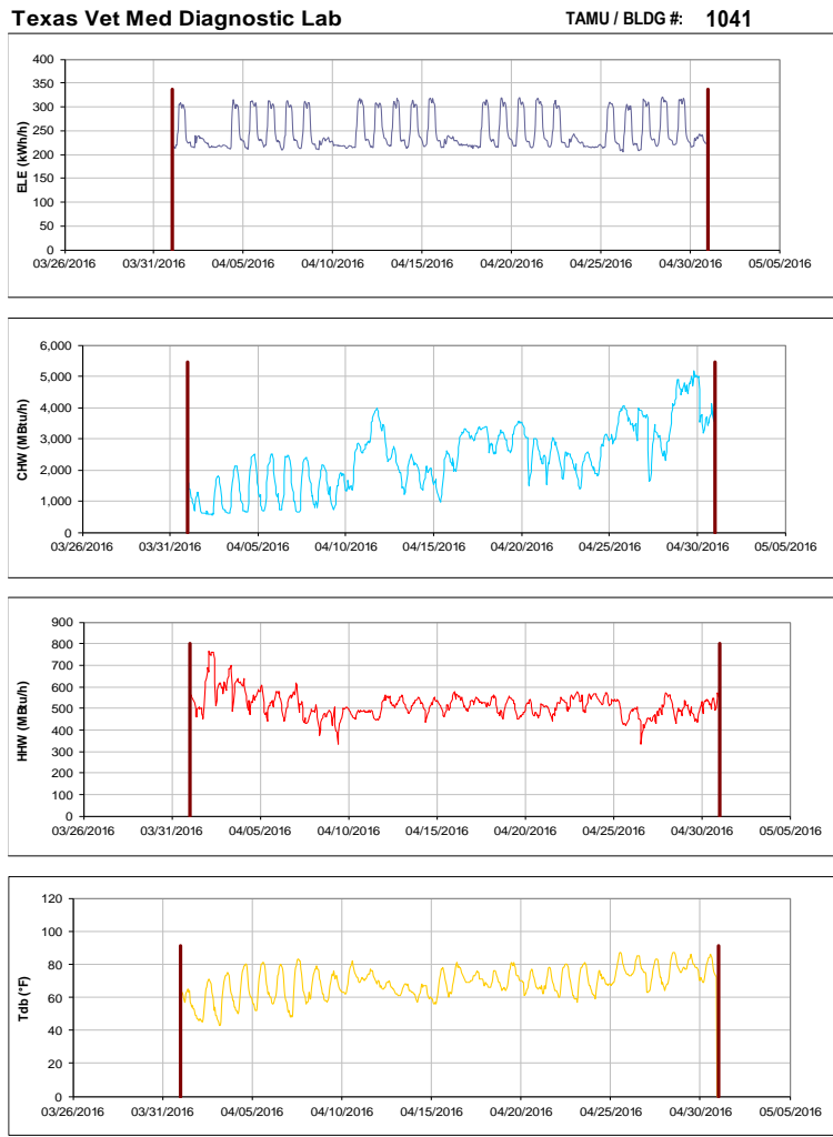
Figure III-123 Hourly Whole Building Electricity, Chilled Water, and Hot Water Consumption for Texas Vet Med Diagnostic Lab during the Month of April 2016 and the Corresponding Hourly Outdoor Dry Bulb Temperature for College Station, TX
