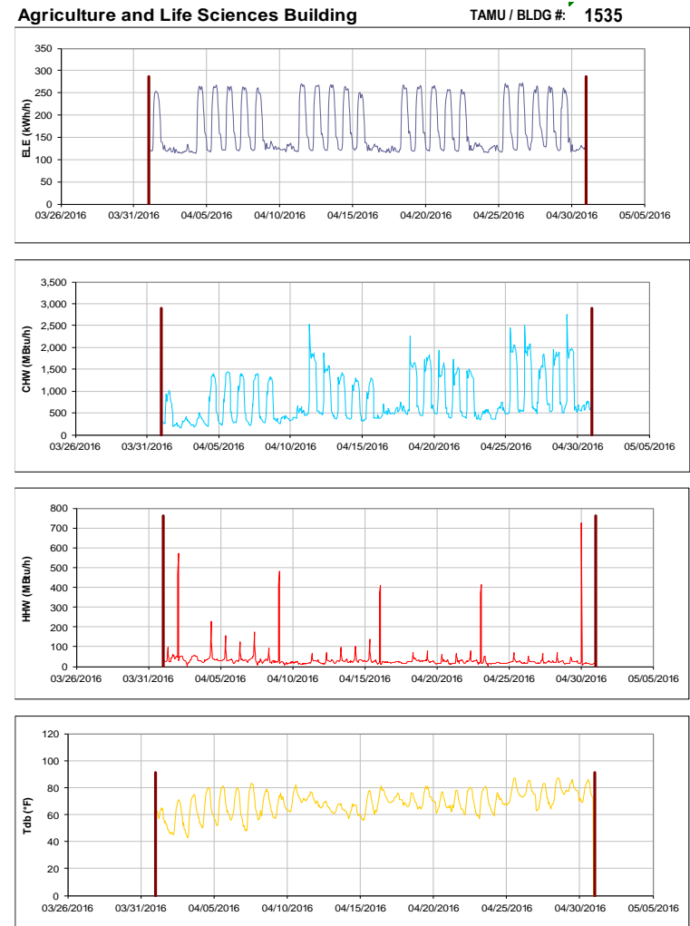
Figure III-160 Hourly Whole Building Electricity, Chilled Water, and Hot Water Consumption for Agriculture and Life Sciences Building during the Month of April 2016 and the Corresponding Hourly Outdoor Dry Bulb Temperature for College Station, TX
