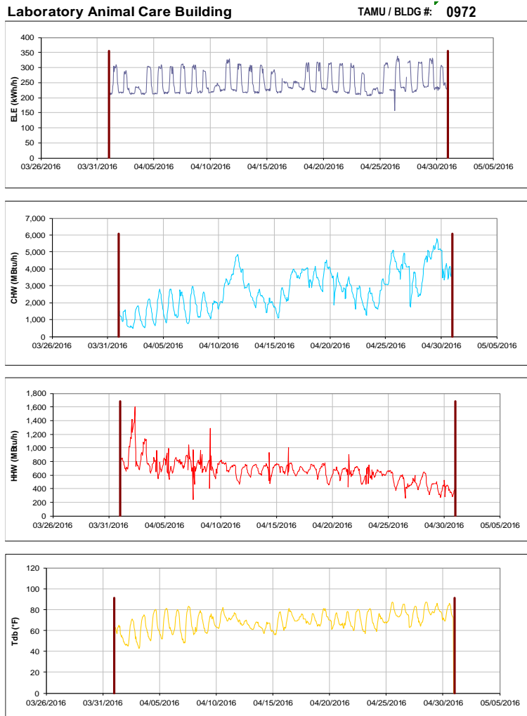
Figure III-121 Hourly Whole Building Electricity, Chilled Water, and Hot Water Consumption for Laboratory Animal Care Building during the Month of April 2016 and the Corresponding Hourly Outdoor Dry Bulb Temperature for College Station, TX
