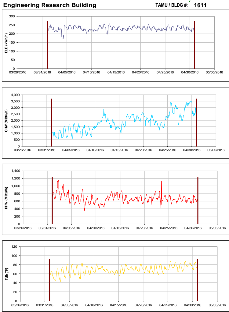
Figure III-179 Hourly Whole Building Electricity, Chilled Water, and Hot Water Consumption for Engineering Research Building during the Month of April 2016 and the Corresponding Hourly Outdoor Dry Bulb Temperature for College Station, TX
