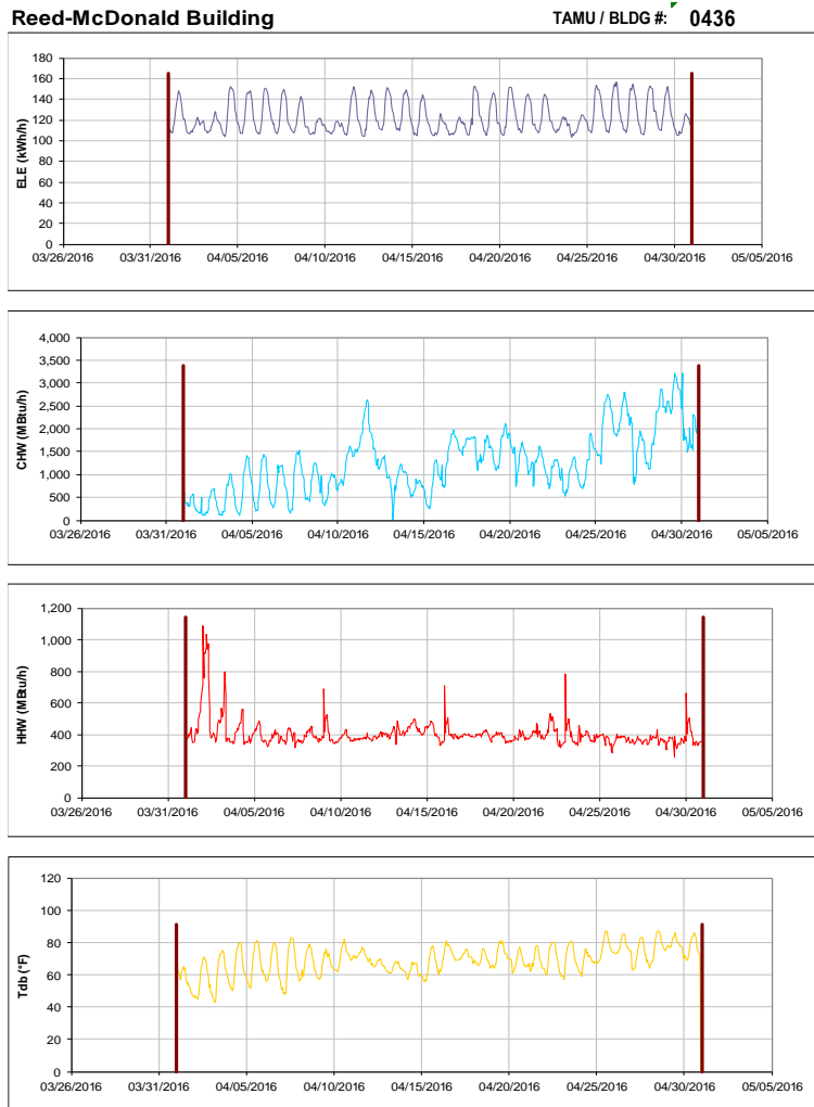
Figure III-55 Hourly Whole Building Electricity, Chilled Water, and Hot Water Consumption for Reed-McDonald Building during the Month of April 2016 and the Corresponding Hourly Outdoor Dry Bulb Temperature for College Station, TX
