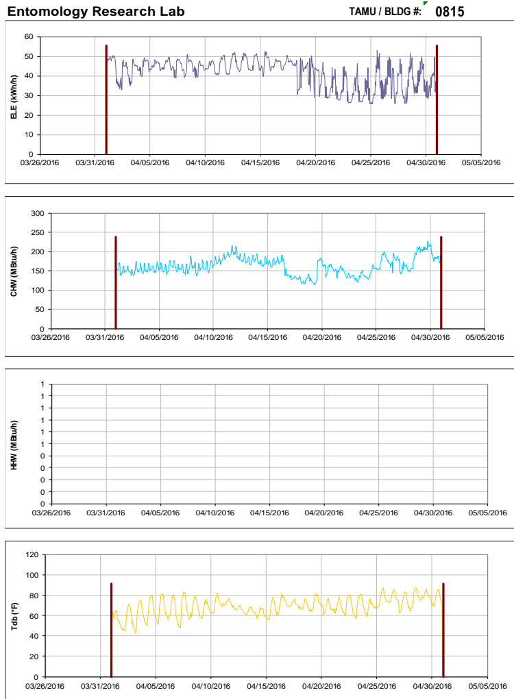
Figure III-119 Hourly Whole Building Electricity, Chilled Water, and Hot Water Consumption for Entomology Research Lab during the Month of April 2016 and the Corresponding Hourly Outdoor Dry Bulb Temperature for College Station, TX
