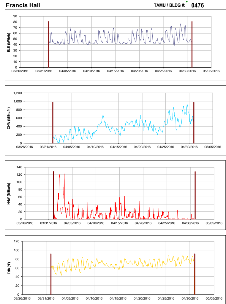
Figure III-86 Hourly Whole Building Electricity, Chilled Water, and Hot Water Consumption for Francis Hall during the Month of April 2016 and the Corresponding Hourly Outdoor Dry Bulb Temperature for College Station, TX
