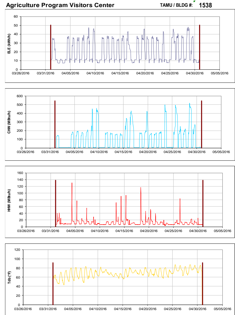
Figure III-162 Hourly Whole Building Electricity, Chilled Water, and Hot Water Consumption for Agriculture Program Visitors Center during the Month of April 2016 and the Corresponding Hourly Outdoor Dry Bulb Temperature for College Station, TX
