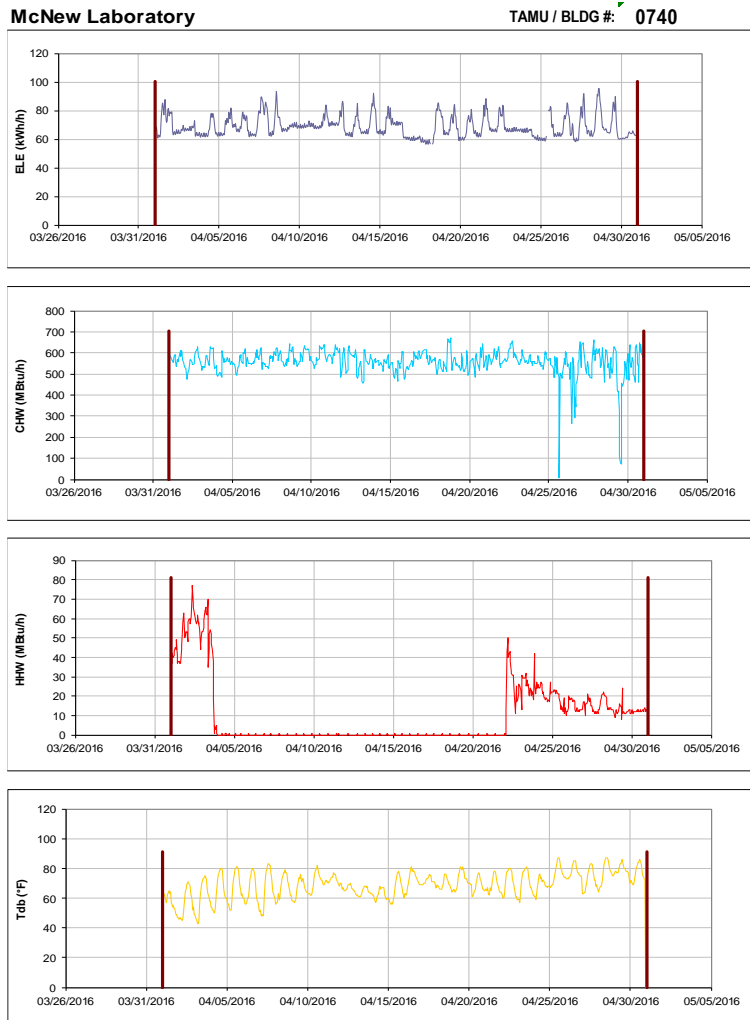
Figure III-117 Hourly Whole Building Electricity, Chilled Water, and Hot Water Consumption for McNew Laboratory during the Month of April 2016 and the Corresponding Hourly Outdoor Dry Bulb Temperature for College Station, TX
