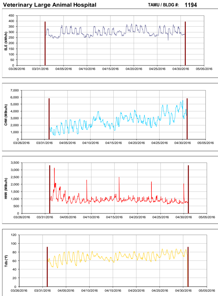
Figure III-129 Hourly Whole Building Electricity, Chilled Water, and Hot Water Consumption for Veterinary Large Animal Hospital during the Month of April 2016 and the Corresponding Hourly Outdoor Dry Bulb Temperature for College Station, TX
