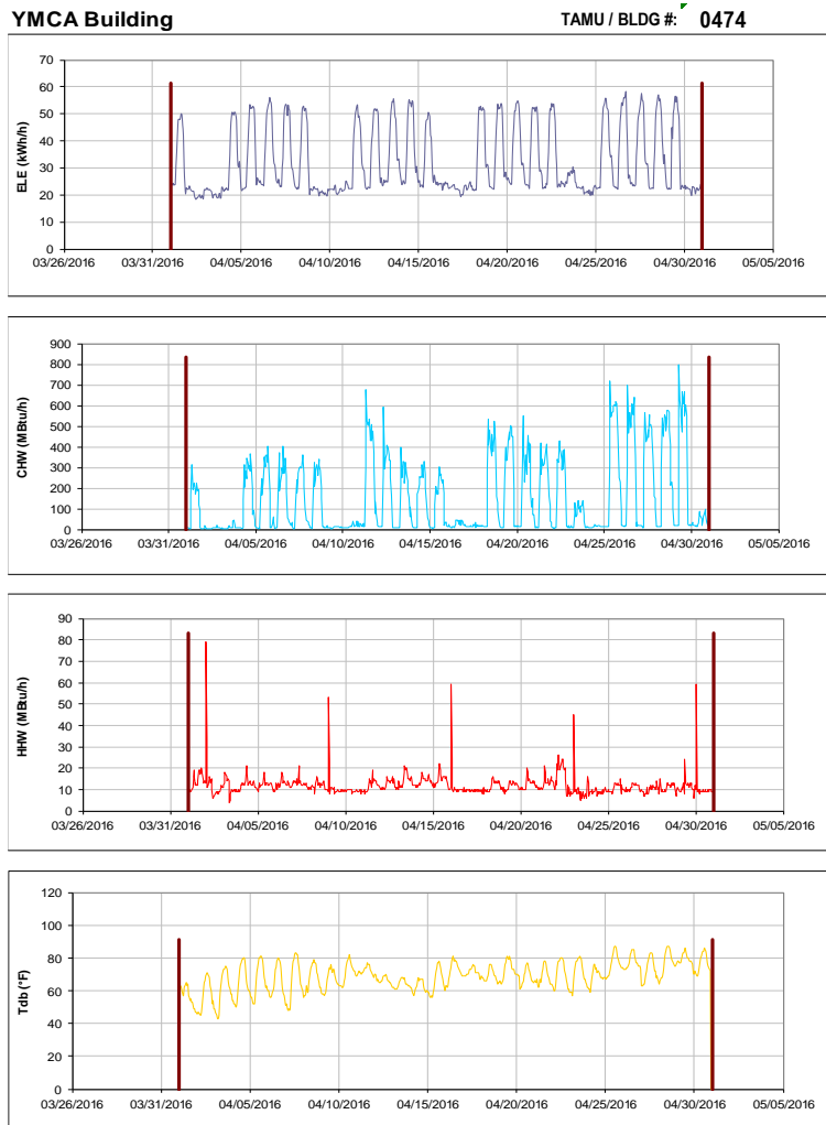
Figure III-85 Hourly Whole Building Electricity, Chilled Water, and Hot Water Consumption for YMCA Building during the Month of April 2016 and the Corresponding Hourly Outdoor Dry Bulb Temperature for College Station, TX
