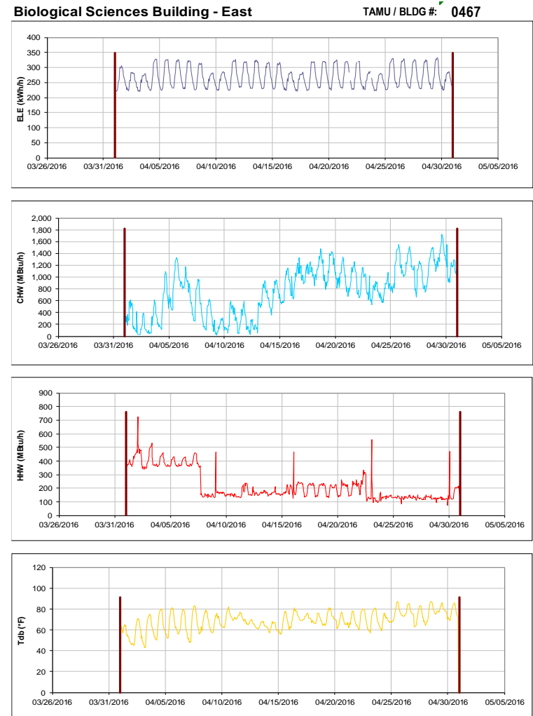
Figure III-78 Hourly Whole Building Electricity, Chilled Water, and Hot Water Consumption for Biological Sciences Building - East during the Month of April 2016 and the Corresponding Hourly Outdoor Dry Bulb Temperature for College Station, TX
