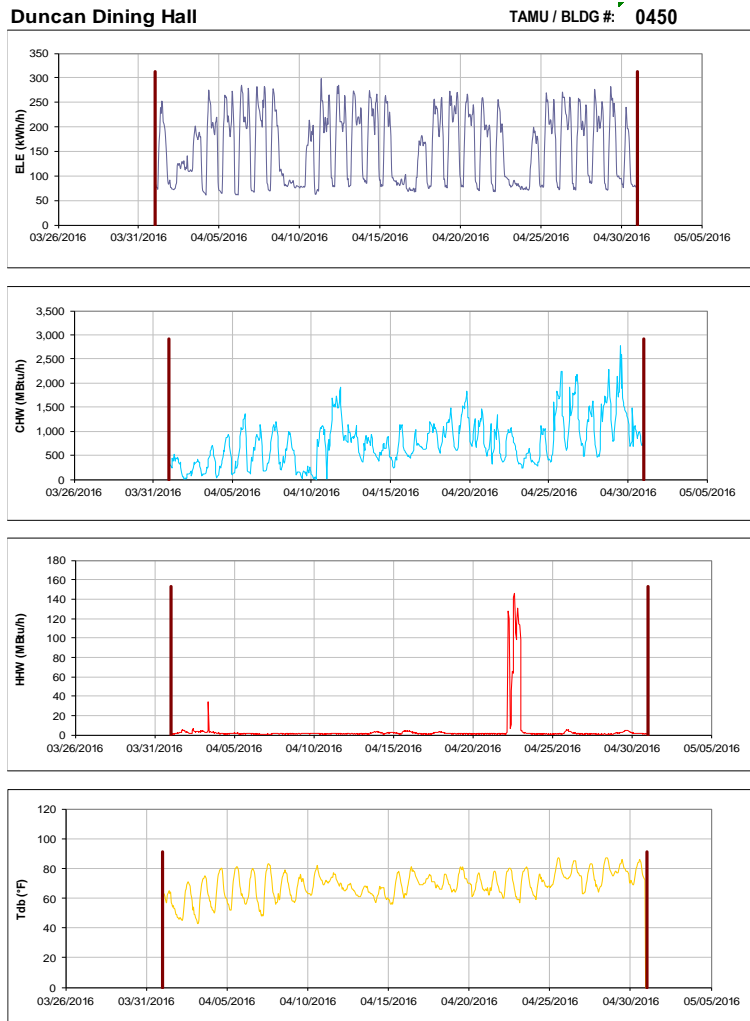
Figure III-69 Hourly Whole Building Electricity, Chilled Water, and Hot Water Consumption for Duncan Dining Hall during the Month of April 2016 and the Corresponding Hourly Outdoor Dry Bulb Temperature for College Station, TX
