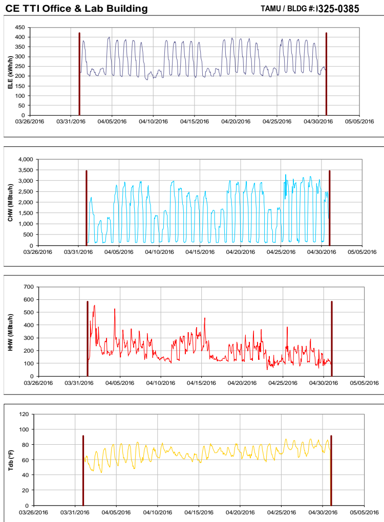
Figure III-9 Hourly Whole Building Electricity, Chilled Water, and Hot Water Consumption for CE TTI Office & Lab Building during the Month of April 2016 and the Corresponding Hourly Outdoor Dry Bulb Temperature for College Station, TX
