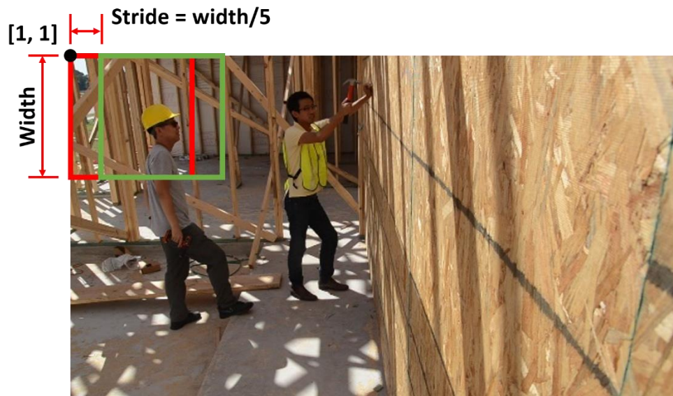
Figure 31 Illustration of sliding window. The sliding window starts from the origin point [1, 1] located at the upper left corner of the image. The red square represents the first window. The window moves every stride size, and the green square represents the second window. The sliding window keeps moving vertically and horizontally until its lower right corner reaches the lower right corner of the testing image.
