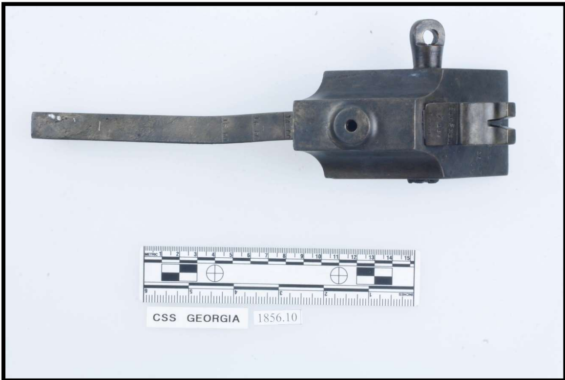
FIGURE 5.15. CSSG 1856.10 - Assembled Tangent Sight (photo by author).
