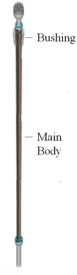
Figure 4 3D drawing of the TSJ. Reprinted from (RTI Energy Systems 2005)
