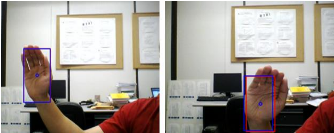
Figure 16. Captures of tracking implementation on the movement of a hand. Kalman filter (red box) continuously records the correct position of the center of window
