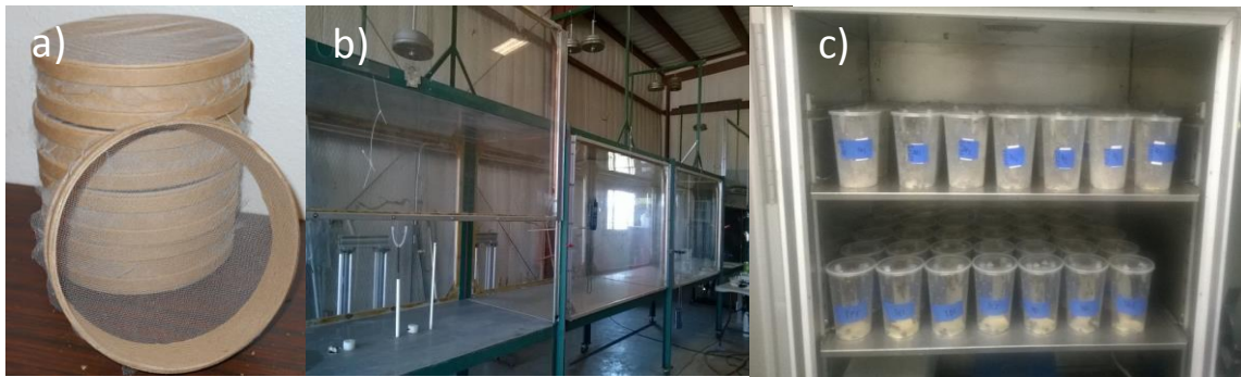
Figure C-1. Experimental set up used to test the effects of pesticides on honey bee forager survival. First, a) about 30-40 bees were loaded into clean bioassay cages. Then, b) cages were placed in a wind tunnel and exposed to either a pesticide-free control or pesticide-laden treatment in increasing concentrations as shown in Tables 2, 3, and 4. Once treated, the caged bees were transferred into c) plastic holding units with feeders containing 50:50 sucrose solution ad libitum and placed in an incubator held at 34°C to measure worker mortality every 24 h for 10 days.
