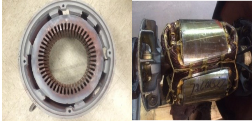
Fig 2.20: SG stator (left) and rotor (right) prototype.
