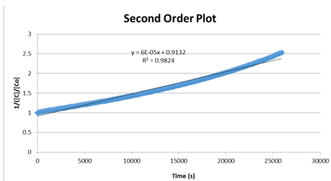
Figure 43: Second Order Plot from IPO Experiment on GDI E0 PM at 440°C (Left)
