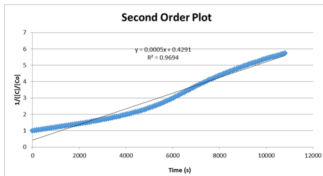
Figure 31: Second Order Plot from IPO Experiment on GDI E0 PM at 490°C
