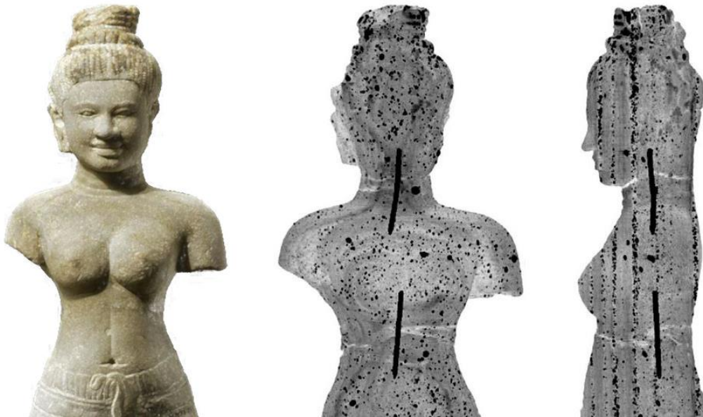
Figure 5.14: CT scan of the Khmer sandstone statue [14].
