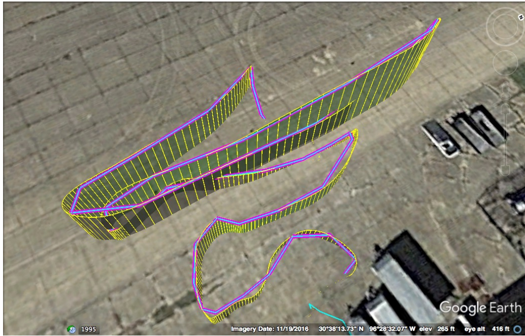
Figure 5.5: Flight path of the F450 as recorded by the autopilot (yellow), Slash (cyan), and F450 (magenta)
