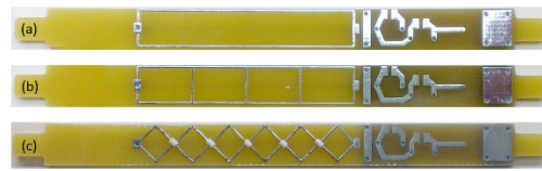
Figure 2. Trace-only DPP-like coils without any capacitors. These coils were built to validate the induced current being cancelled on the return paths of the DPPX coil. (a) Dual plane pair. (b) Dual plane pair with shorted return paths. (c) Dual plane pair with criss- cross return paths.
