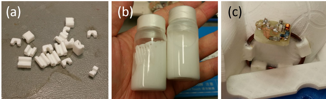
Figure 50. Using coil clips and PLA cement to help assemble coil arrays on a coil former of irregular shape in a space-restricted environment. (a) 3D printed coil clips made of PLA material. (b) PLA cement made by dissolving recycled PLA material in tetrahydrofuran solvent. (c) A coil mounted on the coil former by fusing coil clips with tetrahydrofuran. The gaps between the coil and the coil clips were filled with PLA cement. As is demonstrated in (c), all components except the phase shifter were able to be soldered on the coil before the coil was mounted on the coil former, because of the streamlined circuit design. This negated the need to solder small components in confined spaces.
