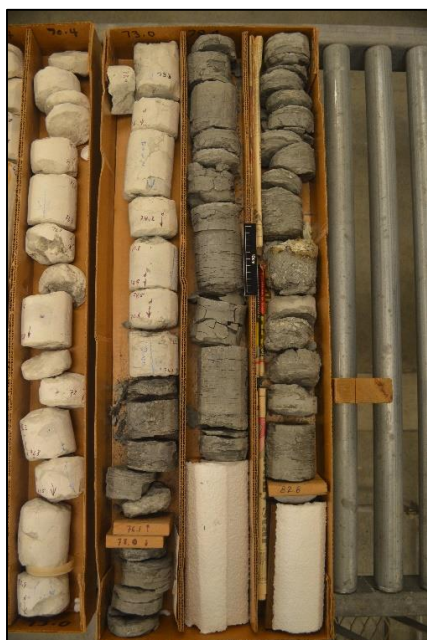
Figure B-2. Photo of whole Laughlin AFB core. Showing contact of the white colored Buda Formation with the dark grey Del Rio Formation
