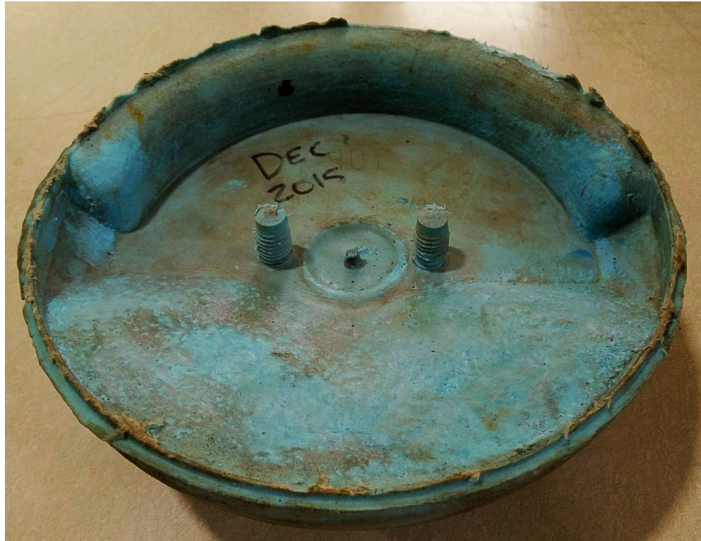
Figure 4.8: Silicone mold of the clearance volume: view of the piston crown
