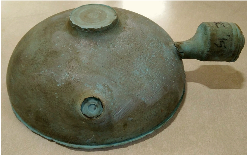
Figure 4.7: Silicone mold of the clearance volume: view of the inside of the cylinder head
