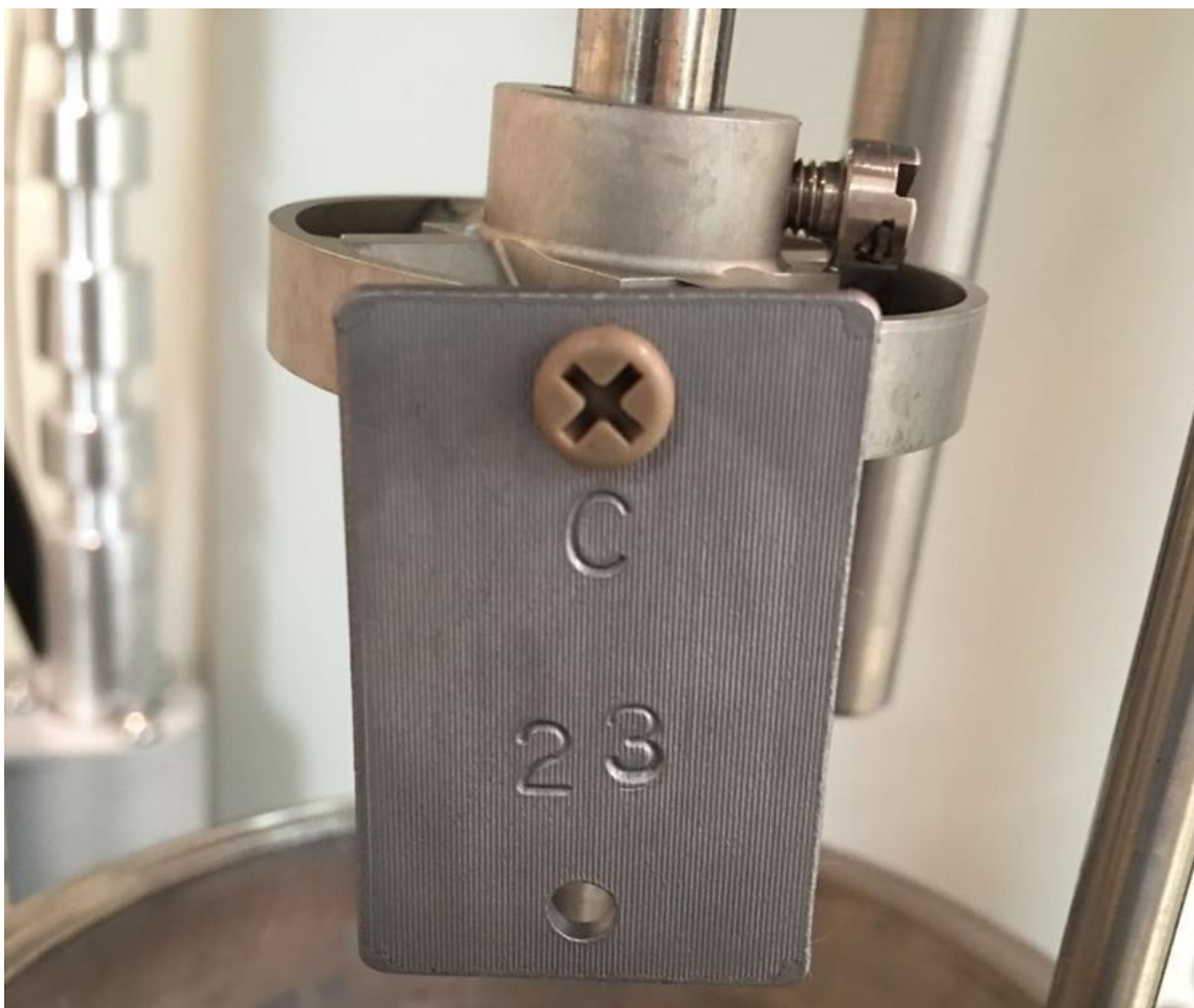
Figure 8: Coupon mounted to rotating shaft of reactor.
