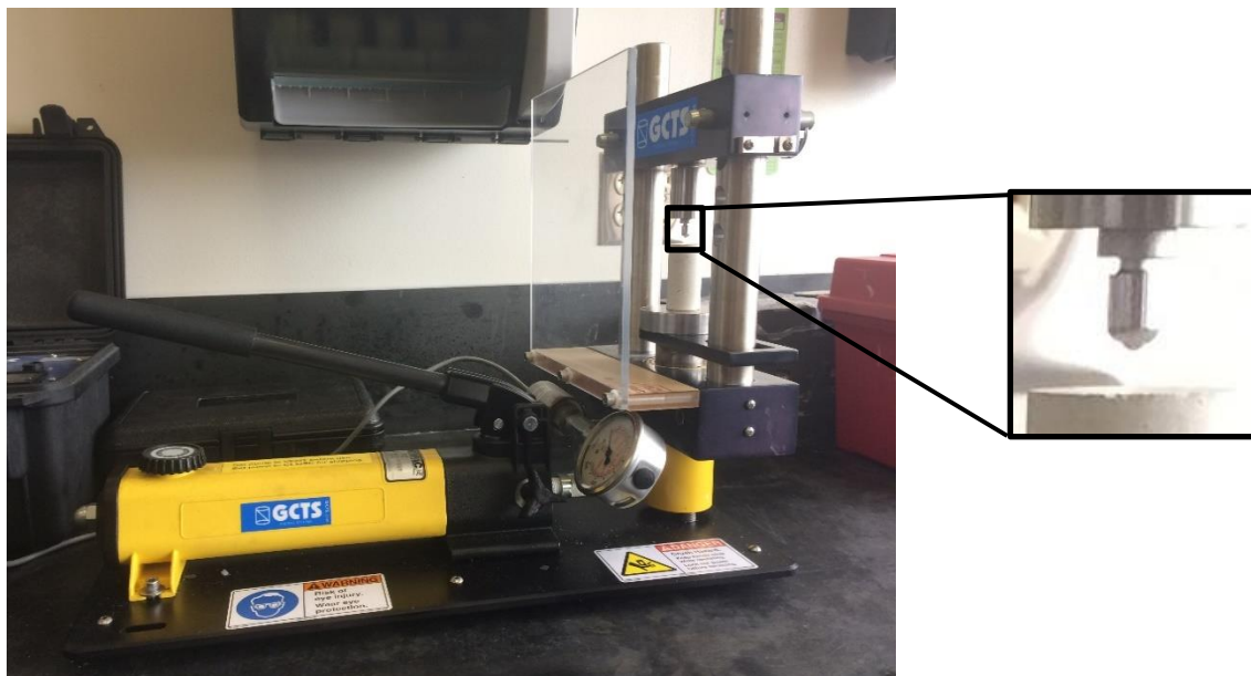
Figure 7-Apparatus for conducting the Brinell hardness test with zoomed in view of the spherical indenter.
