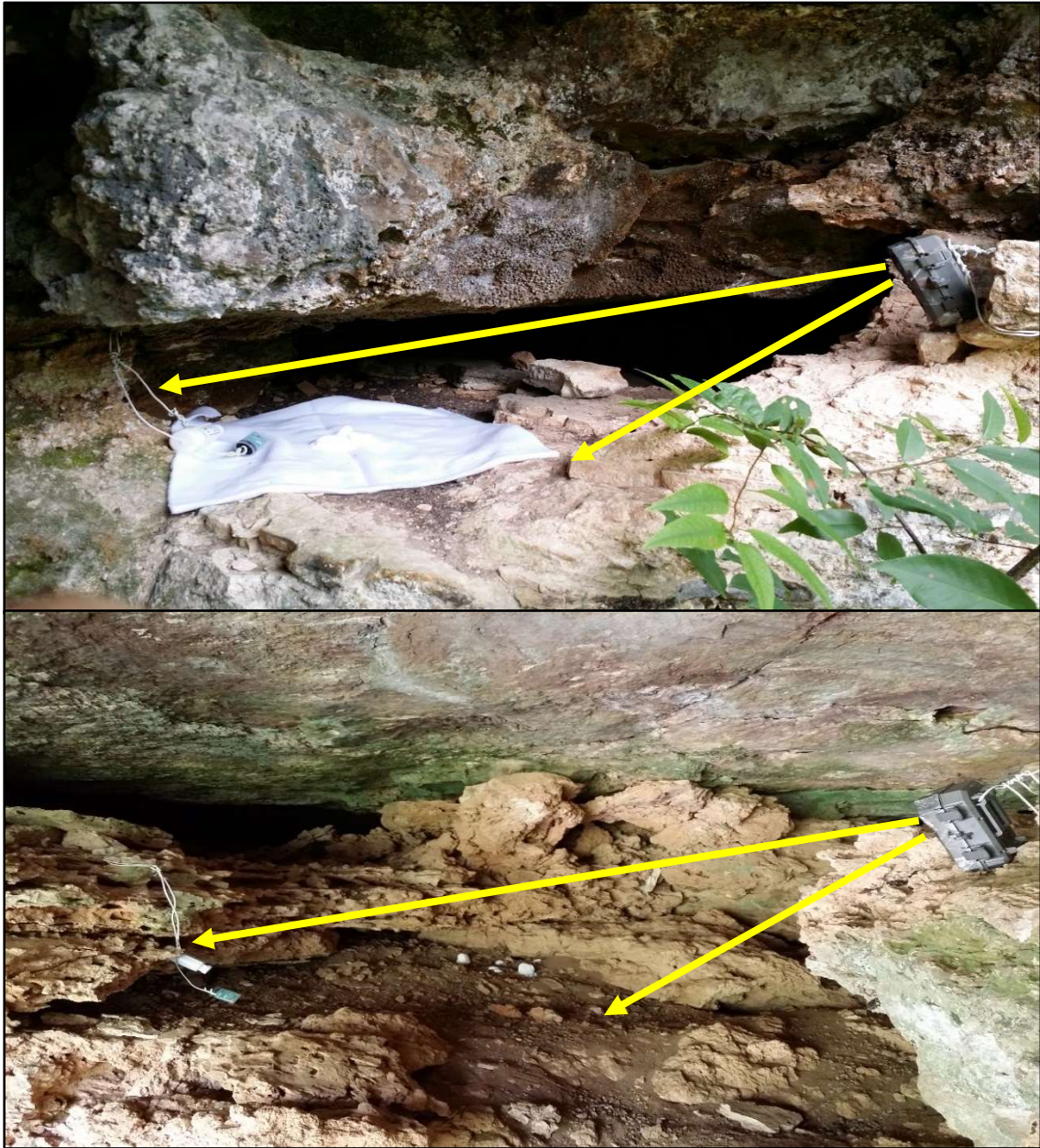
Figure 6. The animal activity collection setup using motion sensor triggered trail camera at the GCSNA, TX. Two trail cameras, Stealth CAM® Model# STC-G42NG (Stealth CAM, LCC, Grand Prairie, TX), were installed at each Ornithodoros turicata -active cave from September 2015 to October 2016. Trail cameras were positioned 1 to 1.5 meters from the tick survey site within the cave to ensure captured images would have full tick survey site in view (indicated by the yellow arrows) as well as animals that may have triggered the trail camera sensors. Top and bottom: Trail camera set up at Little Crevice Cave and Wash Out Cave, respectively.
