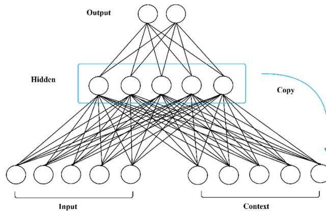
Figure 3. An illustration of Elman’s recurrent neural network.
