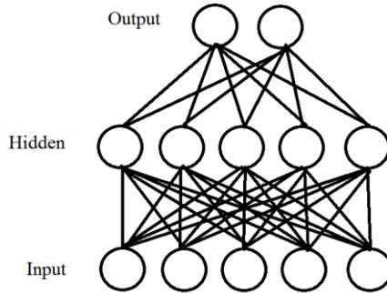
Figure 2. The internal structure of the feedforward neural network used.
