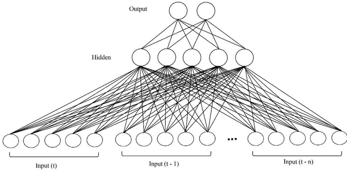
Figure 4. An illustration of a time-delay neural network with the delayed inputs fed into the hidden layer.
