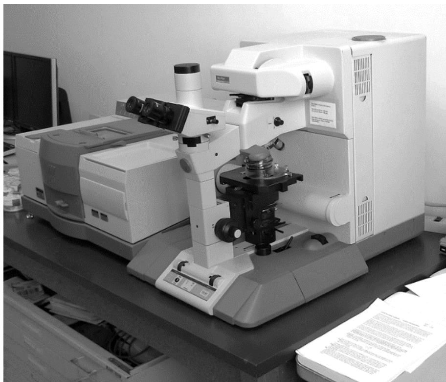
Figure 1. An FTIR bench coupled to an IR microscope. The microscope is cooled to 77 K before collecting measurements. Low temperatures increase the radiation produced by vibrational stretching of polar ions and molecules in the IR, which improves the quality of the spectra by enhancing absorption features characteristic and specific to certain compounds. For quartz in reference to this study, it would be the broad band absorption of OH centered at \sim 3400\text{ cm}^{-1} .
