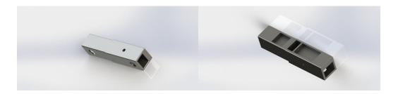
Figure #10. (Left) View of the side where direct access to the mechanical lock (in case of battery failure) is placed. (Right) Overhead view displaying RFID reader, LED, and 9V battery compartments.
