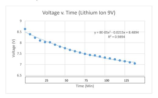
Chart 2. Energizer 9V lithium ion battery voltage v. time test results. 120 minute test period.
