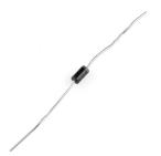
Figure #7. "Fly-back" Schottky Diode
