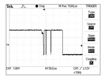
Figure #5. Oscilloscope output of a system without a de-bouncing circuit (note the several dips in the signal output).
