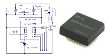
Figure #1. ID-Innovations ID-2LA circuit diagram (Left) and device (Right).
