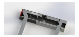
Figure #11: Cross-sectional view displaying the "three-sleeve" design, allowing access to the battery compartment
