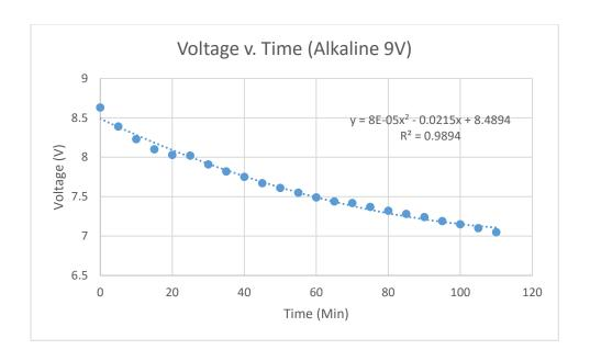
Chart 1. Duracell 9V alkaline battery voltage v. time test results. 120 minute test period.
