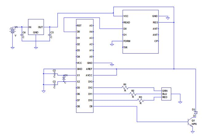
Figure #8. Bicycle breadboard design schematic
