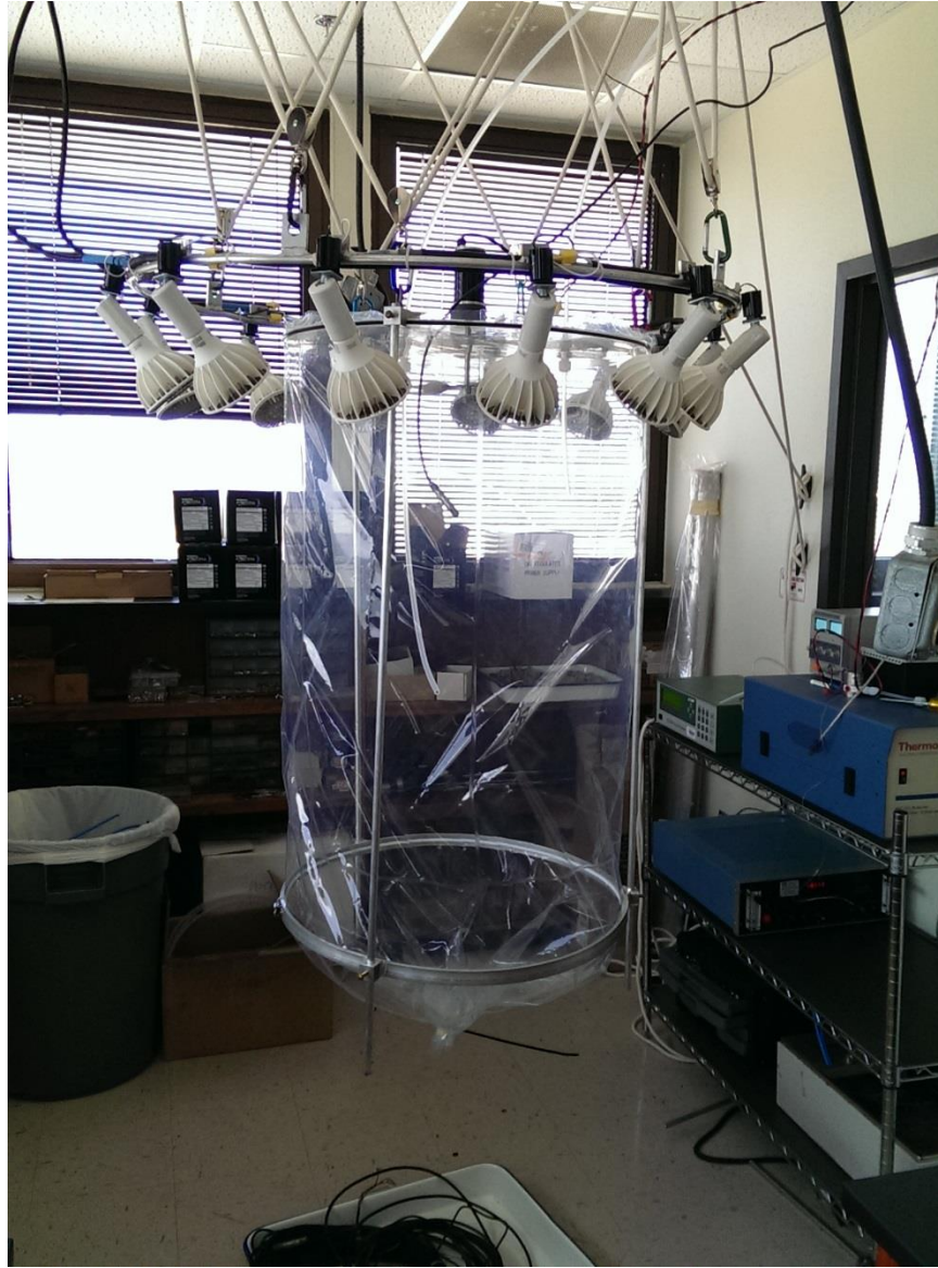
Figure 1. A photo of the completed chamber assembly. The light ring and chamber are suspended by separate pulley systems; note the fan motor above the Plexiglas plate, and the fan blade within the chamber.
