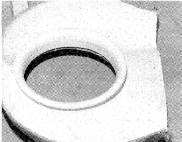
Figure 21. Wall Streamline Traces on Interior of Intake B-1. View of intake half-section including pump entry plane. Flow enters from the right.
