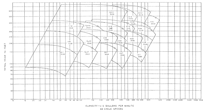
Figure 1. Hydraulic Coverage of a Typical Line of Direct Drive, Single Stage Process Pumps.
