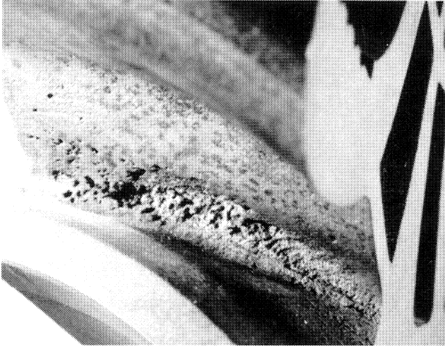
Figure 22. Cavitation Damage along Inlet Vane of a 12 Percent CR Boiler Feedwater Pump.
