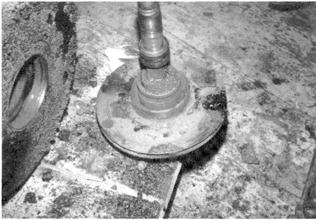
Figure 9. Fatigue Failure of Impeller Due to Turbulent Flows Caused by Several Installation Errors.
