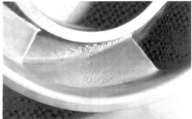
Figure 2. Cavitation Damage on 12 × 18 CA Suction Impeller. The damage accumulated on this impeller occurred over a period of about 18 months operation. It is considered at the end of its operational life. No pressure (or hidden side) damage was observed.
