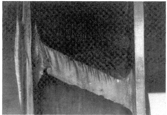
Figure 3. Wear at the Impeller of a Centrifugal Pump.
