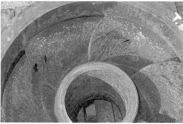
Cast Iron (Pump B): Extensive Damage at Impeller Inlets (Starting at the Shroud Area, Suction Side; Some Damage on Pressure Side). (12 months operation)
