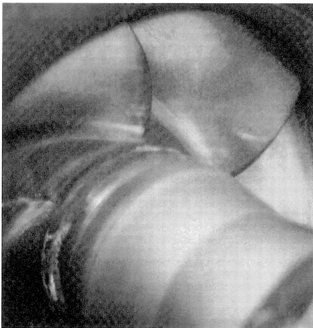
316SS (Pump C): Very Little Damage (Minor Pitting at Blade Inlets, Shroud Area).
