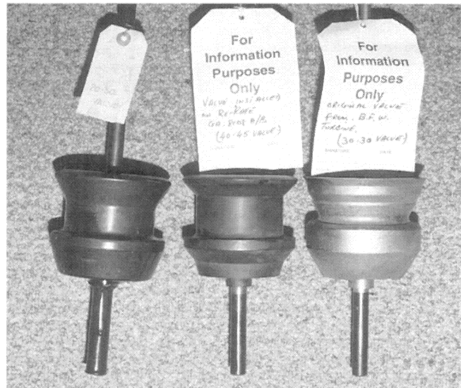
Figure 4. Turbine Governor Valves Left 20-30, Center 40-45, Right 30-30.
