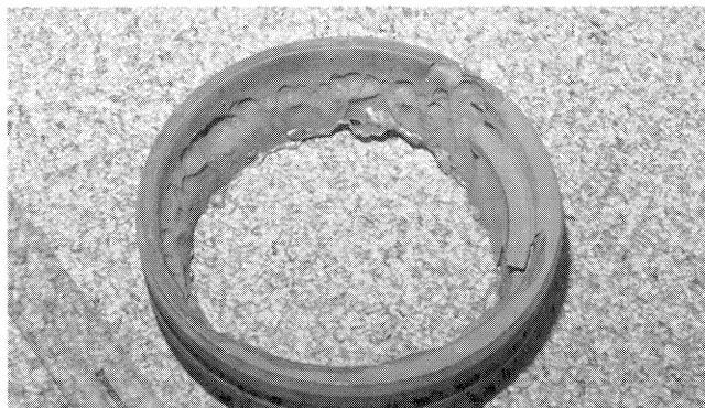
Figure 11. Cavitation Damage to Throttle Bushing Holder (Cut Off End Cover).
