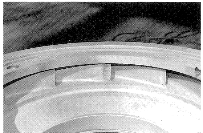
Figure 13. Diffuser Leading Edge Cavitation Erosion.
