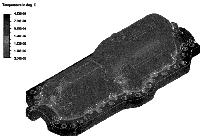
Figure 7. Upward Transient, Temperature Field after t = 16 \text{ min } 30 \text{ sec} .
