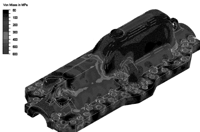
Figure 13. Von Mises Stress on Top Half During Hydrotest Pressure.
