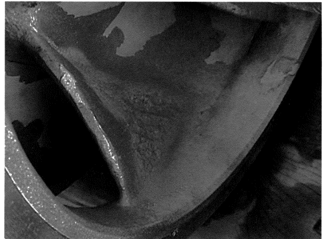
Figure 18. Damage to 316 Stainless Steel Impeller.
