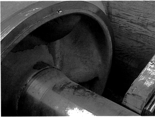
Figure 3. Cavitation Effects on a 316SS Impeller with Ceramic Metal Coating.
