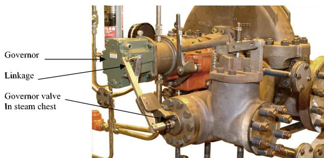
Figure 11. Turbine Controls.
