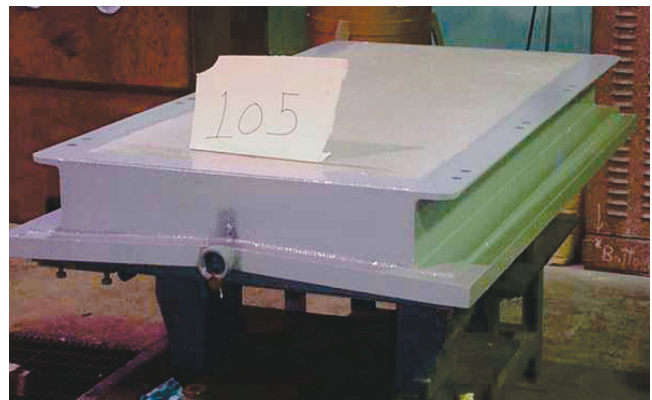
Figure 7. Pregouted Baseplate Bottom.
