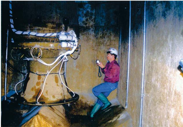
Figure 26. Instrumentation on Pump Housing and in the Sump During Second Test.
