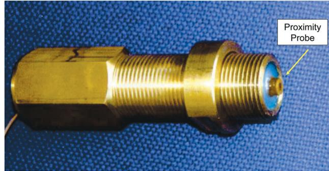
Figure 31. Proximity Probe Installed in Special Probe Holder.
