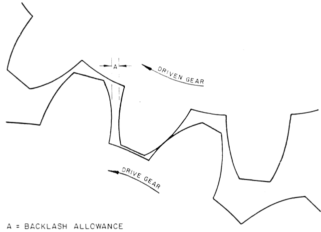
Figure 4a. Gear Tooth Clearance.
