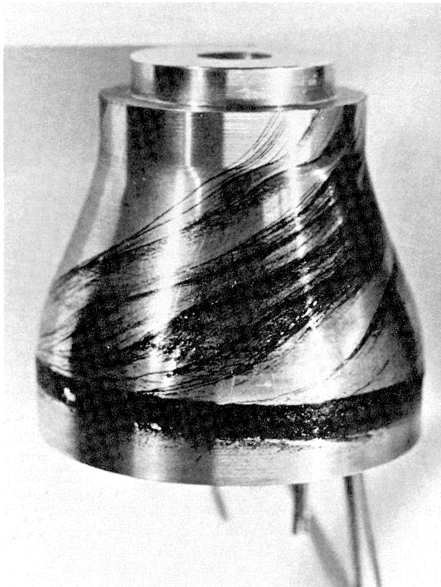
Figure 1. Three Dimensional or Ordinary Separation on a Diffuser Wall Under the Influence of 45° Free Stream Swirling Flow.
