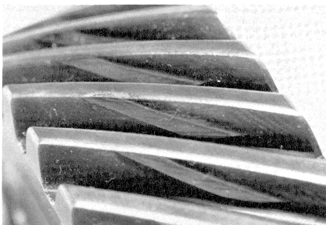
Figure 1b. Centrifuge Gears From Field Test (Six Months Operation on Synthetic Lubricant).
