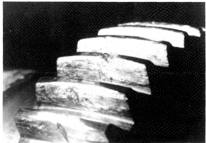
Figure 38. Gear Tooth Failure (inadequate lubrication).
