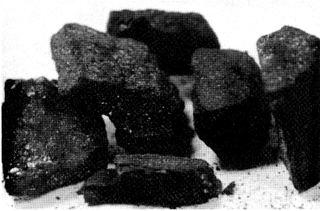
Figure 7. Coked Oil that Blocked Coupling Movements.
