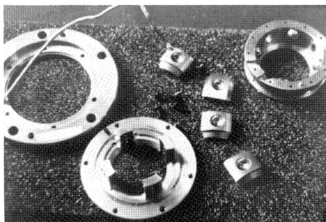
Figure 31. Photograph of New Phase One Compressor-End, Four-Shoe Tilting Pad Journal Bearing Retrofit Showing Spherical Pivots.
