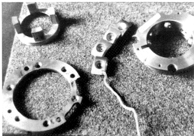
Figure 30. Photograph of New Phase One Expander-End, Four-shoe Tilting Pad Journal Bearing Retrofit Showing Spherical Pivots.
