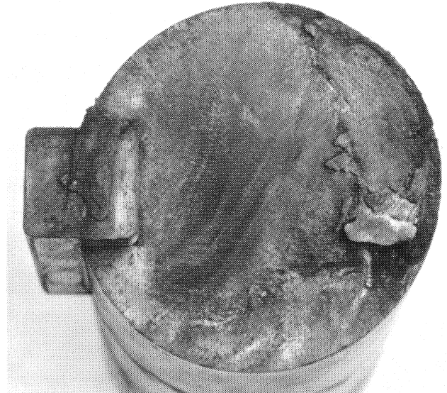
Figure 12. Bending Fatigue Failure of a Pinion Gear Shaft Due to Improper Alignment.
