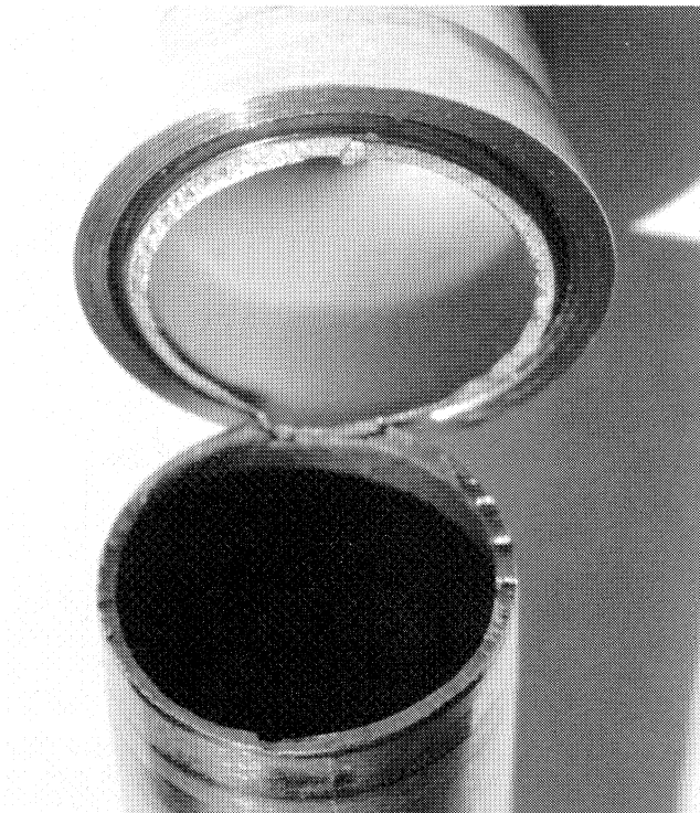
Figure 11. Lube Oil Line Failure due to Overtightening of 1in Tubing Connection. Scoring Initiated Fatigue Fracture.
