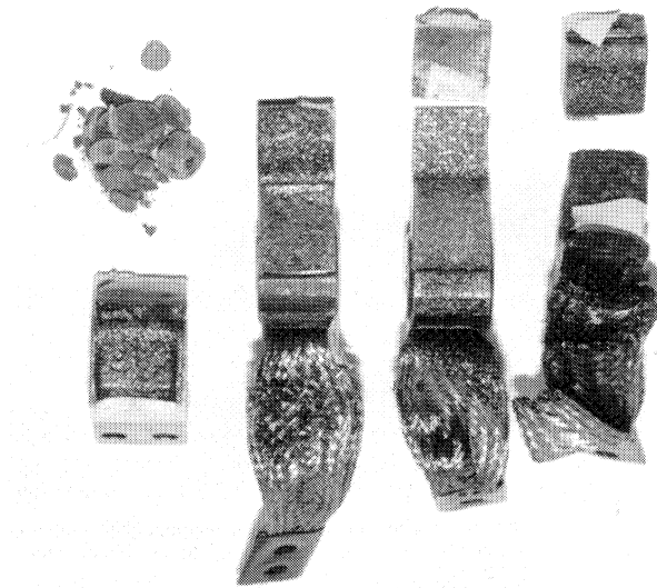
Figure 7. Failures of Transformer Contacts due to Poor Silver Brazing Resulted in Extensive Downtime to the Operating Unit.
