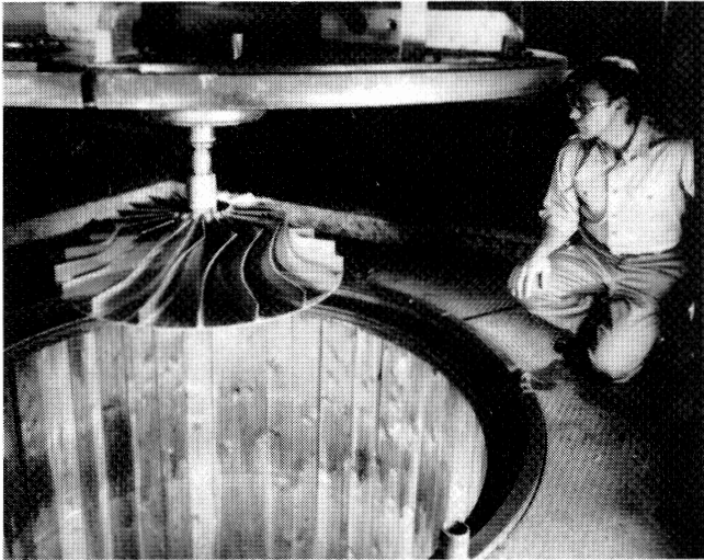
Figure 21. Lowering a Single Stage Impeller into the Overspeed Tip.
