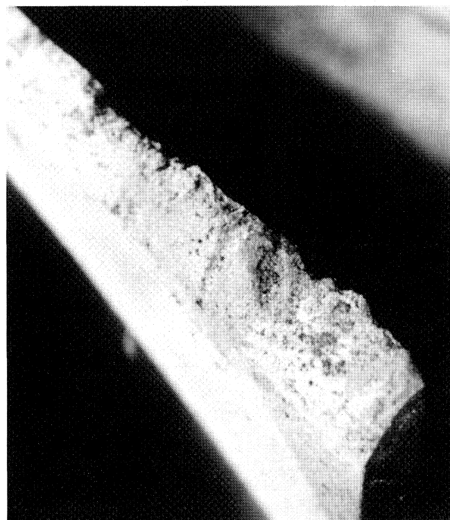
Figure 12. The Eye of a Single Stage Impeller Exhibits the Honeycomb Appearance Characteristic of Corrosion Damage.
