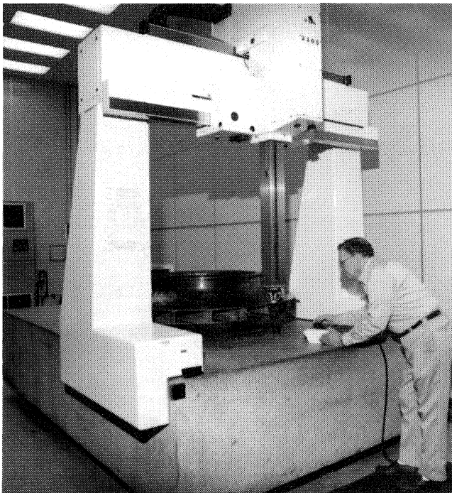
Figure 4. Impeller Flowpath being Measured by Operator on Fixed CMM.
