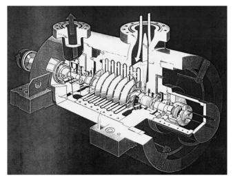
Figure 3. Barrel Compressor Assembly Drawing. (Courtesy Siemans/Demag Delaval)
