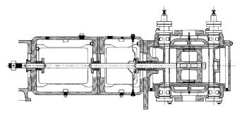
Figure 5. Diagram of a Positive Displacement Compressor Cylinder. (Courtesy Cooper Industries)
