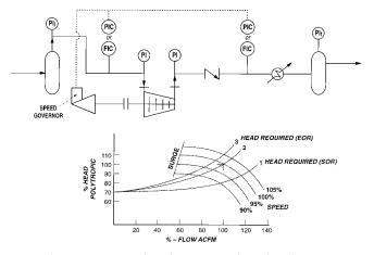
Figure 9. Process Control—Adjusting Head Produced.
