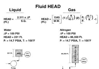
Figure 4. Head Required by the Process for a Pump and a Compressor.
