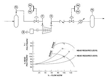
Figure 8. Process Control—Adjusting Head Required.
