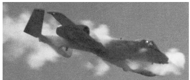
Figure 14. Fairchild A-10 “Warthog” Aircraft with Gatling Gun Firing (3000 Rounds/Minute) Showing Used Propellant Being Ingested into the T-34 High Bypass Turbofans Causing Severe Compressor Fouling.
