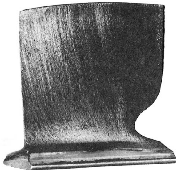
Figure 39. Highly Eroded Compressor Stator Blade.
