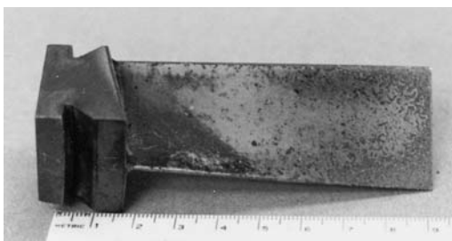
Figure 35. Axial Compressor Blade with Coating Erosion.
