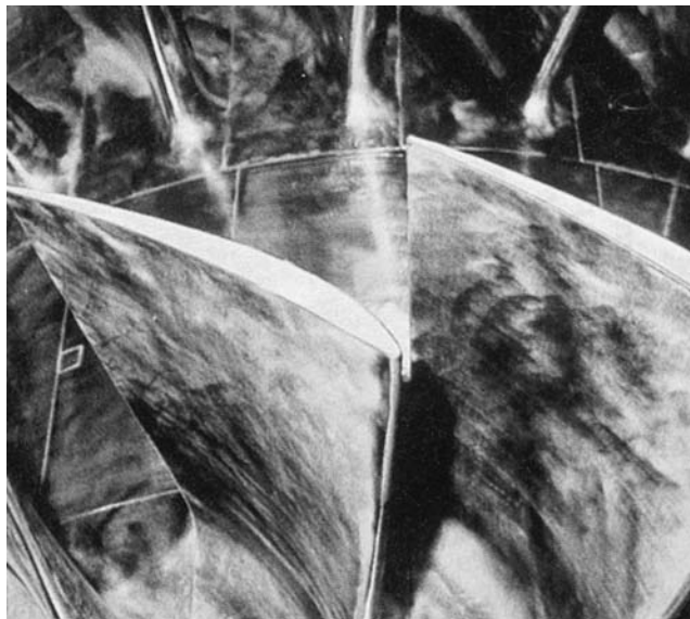
Figure 37. Fouled Turbine Blading.
