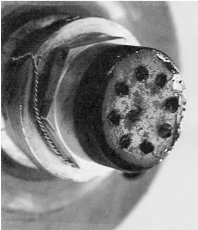
Figure 47. Blocked Fuel Nozzle.
