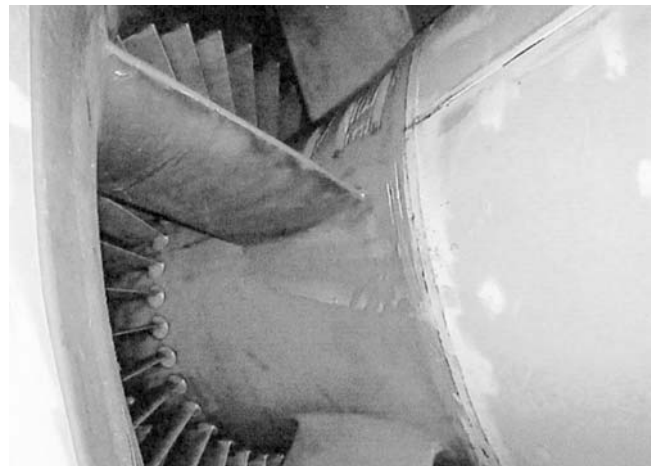
Figure 13. Fouled Intake Strut.
