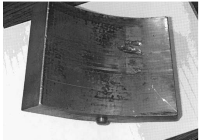
Figure 29. Mechanical Fatigue on a Center Pivot Pad.
