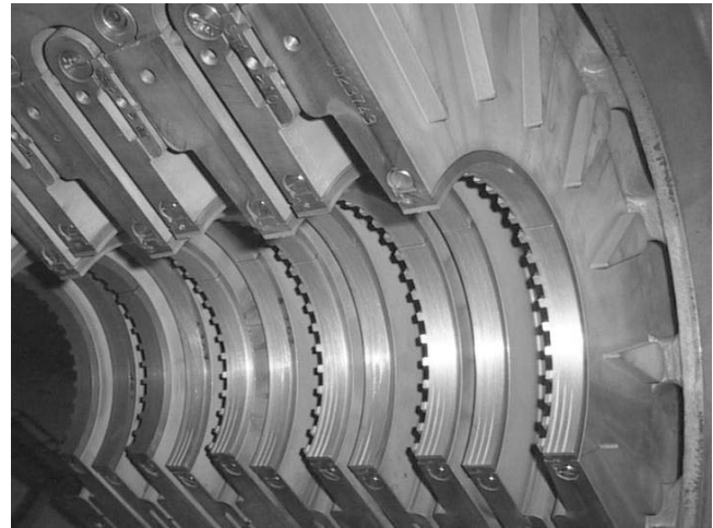
Figure 25. HP Stator and Labyrinth Seals.
