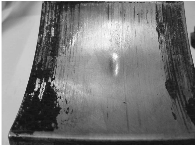
Figure 43. One of the Lower NDE Bearing Pads Showing Dimple Where Babbitt Failed above RTD.
