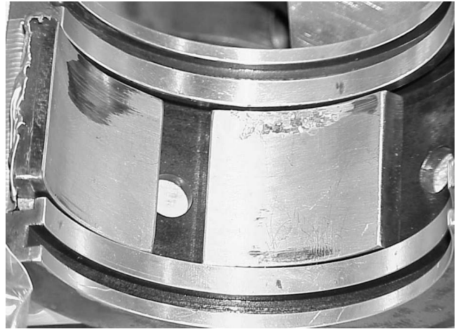
Figure 24. Damaged Radial Bearing.
