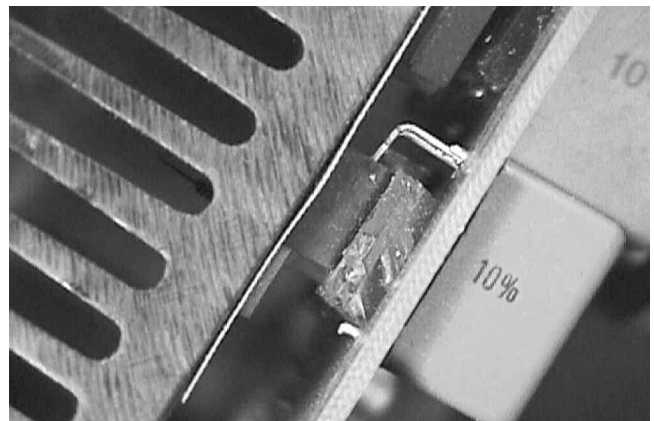
Figure 9. Spacer in Good Condition Holding Integrated Circuit Chip Against Heat Sink.
