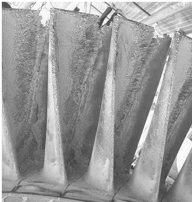
Figure 15. Rotor Blade Primary Erosion.
