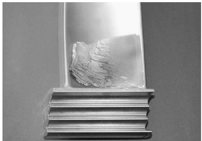
Figure 12. Rotor Blade Deposit Found During Shutdown.
