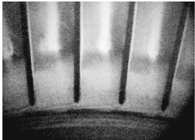
Figure 11. Online Photograph Showing Deposit Formation at Base of Rotor Blade.
